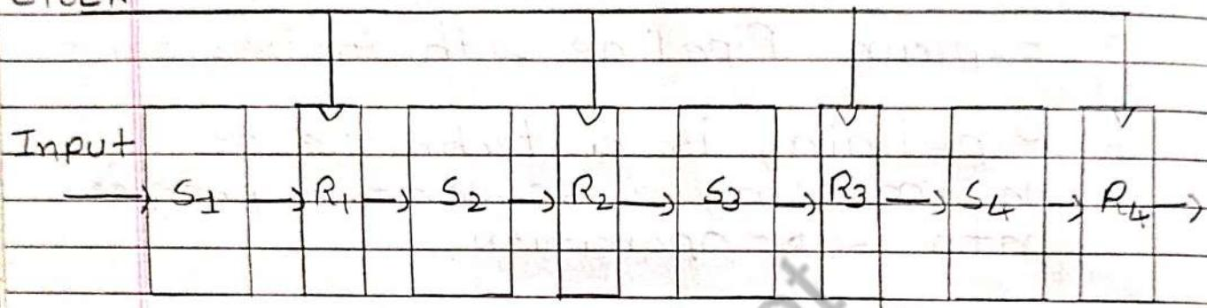
Here,  $R_1, R_2, R_3$  and  $R_4$  are input Register and  $S_1, S_2, S_3$  and  $S_4$  and segment.
